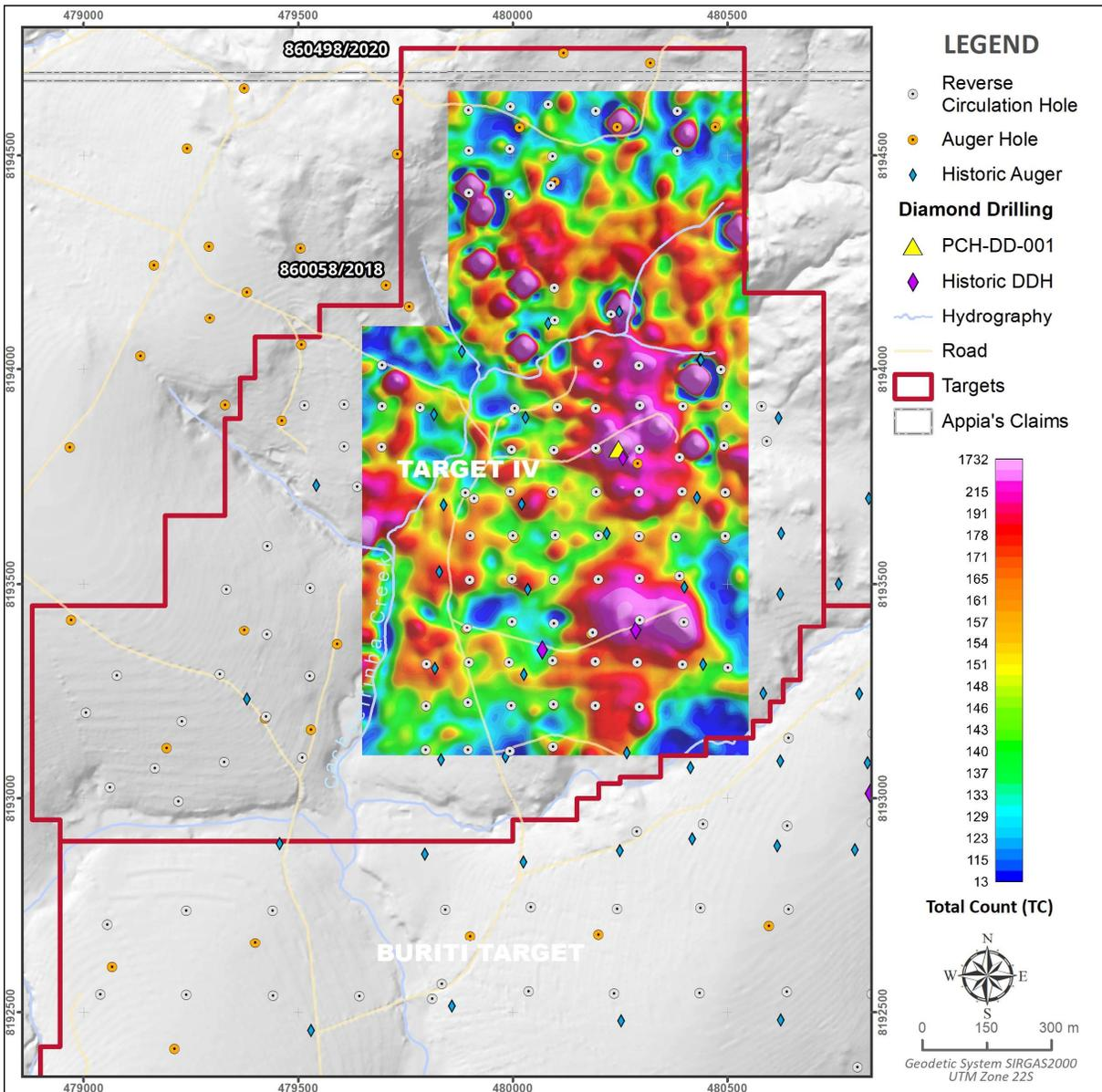
**Figure 6-3 Th Radiometric Signal at Target IV**
